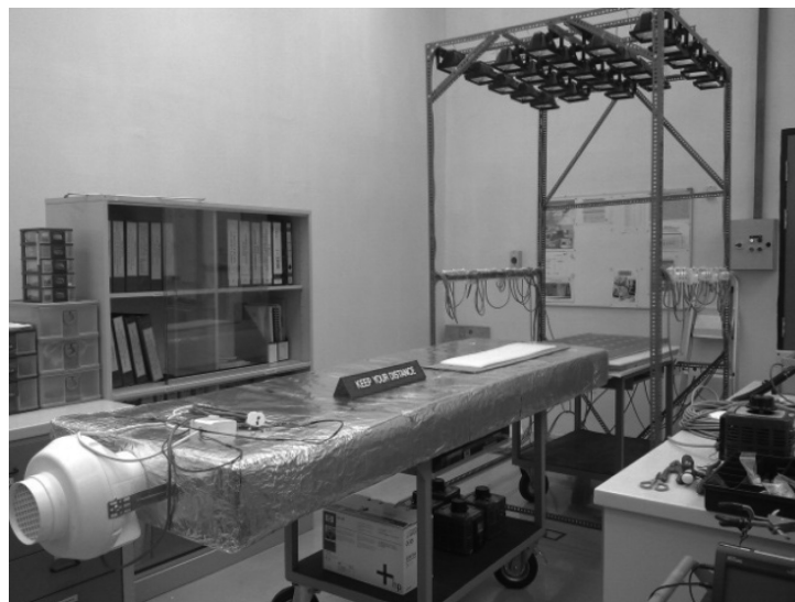
FIGURE 1. The fabricated PV/T solar collector
