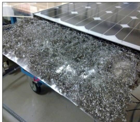
FIGURE 6. PV/T collector with stainless steel wool heat exchanger
